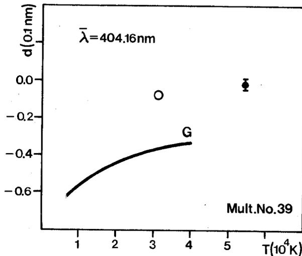
**Fig. 3.** Theoretical Stark shift ( $d$ ) dependence on the electron temperature scaled to the electron density of a  $1 \times 10^{23} \text{ m}^{-3}$ ,  $\bullet$ , our experimental results and those of other authors:  $\circ$ , Djeniže *et al.* (1992). Theory:  $-$ , semiclassical electron impact shifts ( $G$ ) after Griem (1974). The error bars include the uncertainties of the shift and electron density measurements.  $\bar{\lambda}$  is the mean wavelength for the multiplet.
